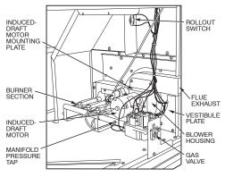
Fig. 27 - Burner Section Details
